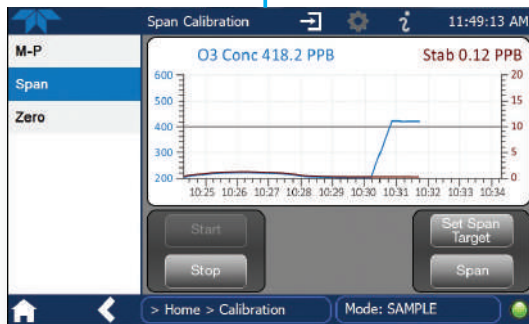
Graphs of zero, span and multi-point calibrations
